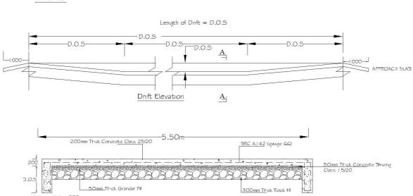
Drift Cross Section A-A
