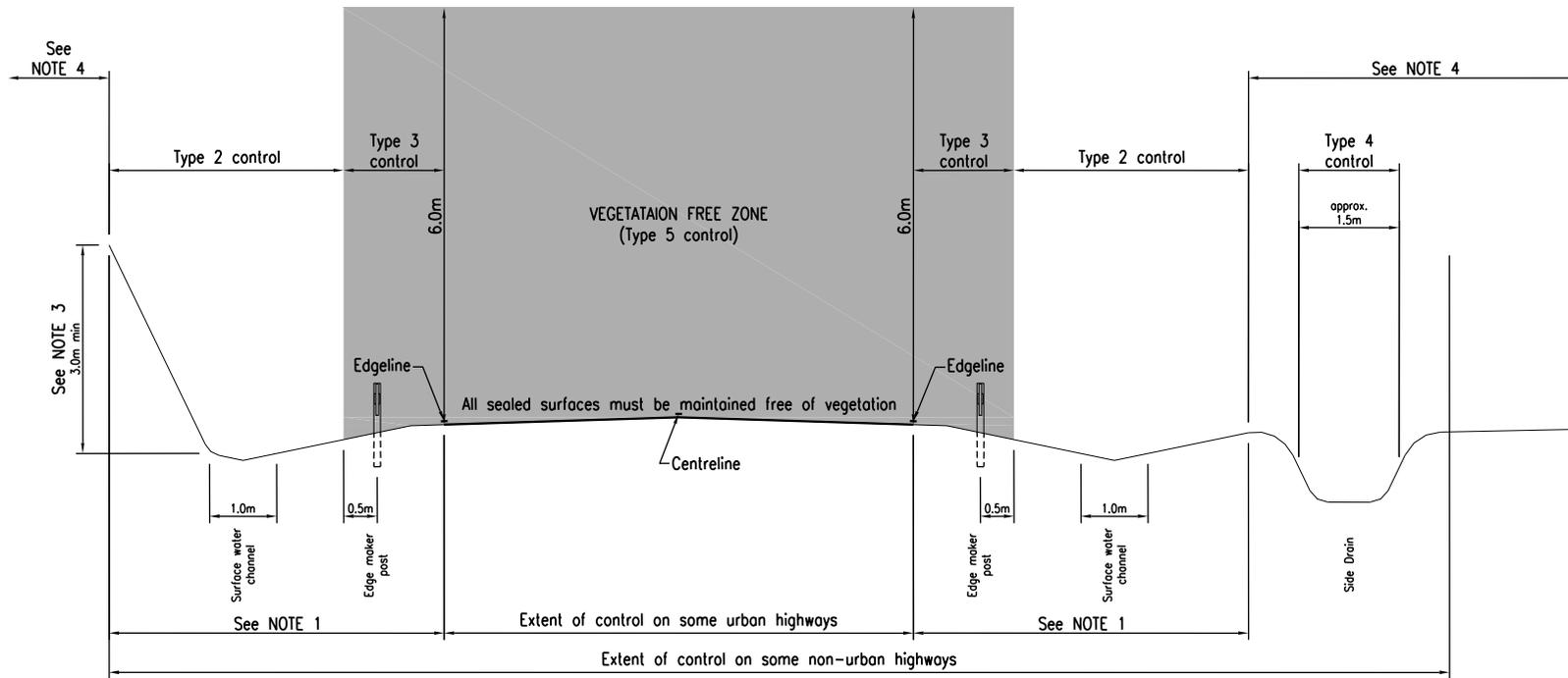
NOTE 1 this distance must be a minimum of 3.0m on straights and on the outside of curves and a minimum of 5.0m on the inside of curves.
