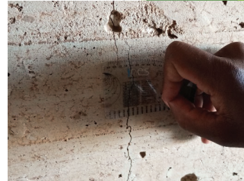
Crack width measurement using a scale
