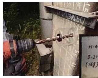
Sampling for Chloride Ion Content Test
