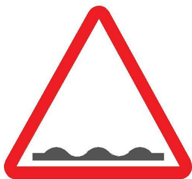
Rumble Strip Sign
